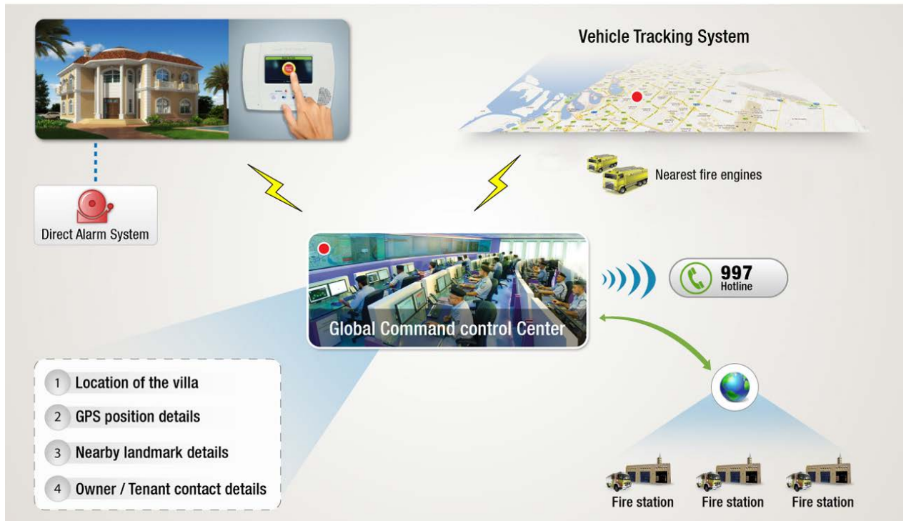
Dubai Civil Defence 24x7 Direct Alarm System operations for homes
